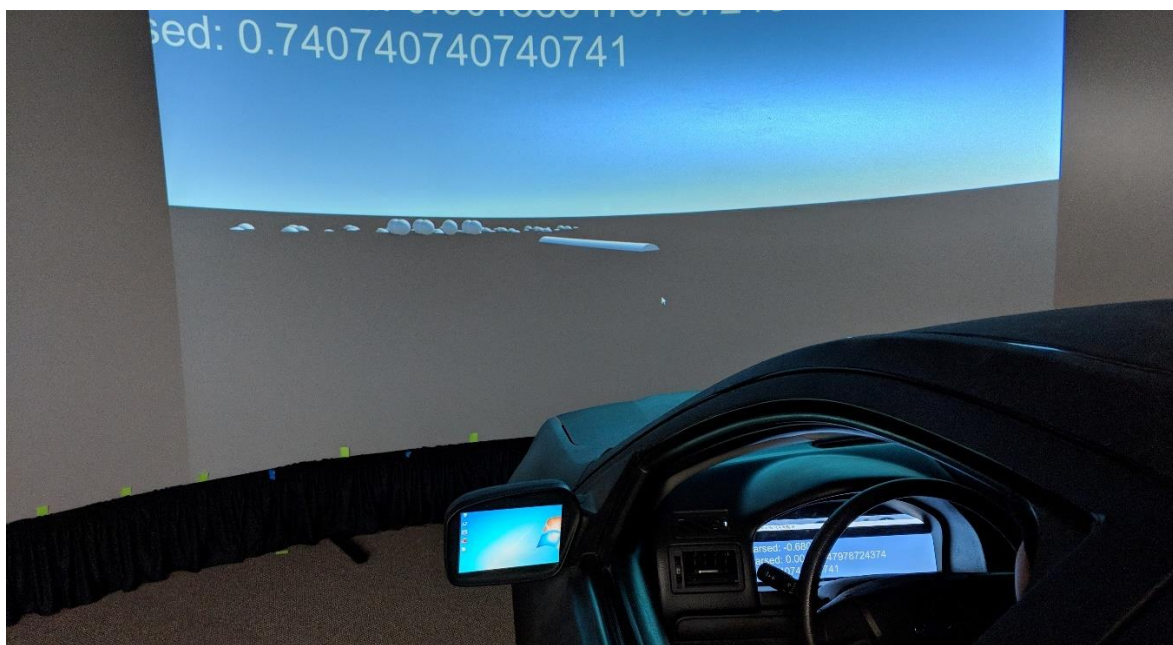
Figure 3. Integration of Unity-based simulator and RTI vehicle cabin
